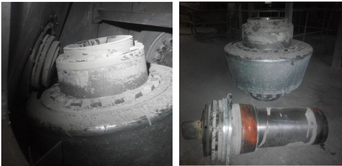
Gambar.5 Shaft Roller patah
