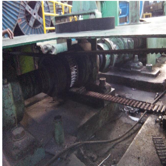
Gambar 3.1.2 Timing Belt Rusak
