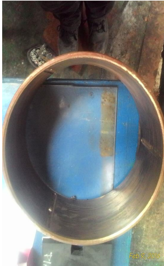
Gambar.4 Bantalan connecting rod berbahan bronze
