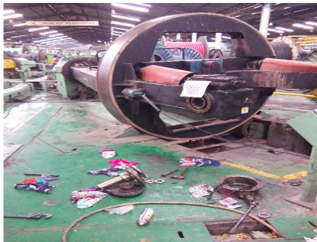
Gambar 4.1 kerusakan HAR2000 (Bobbin jatuh)
